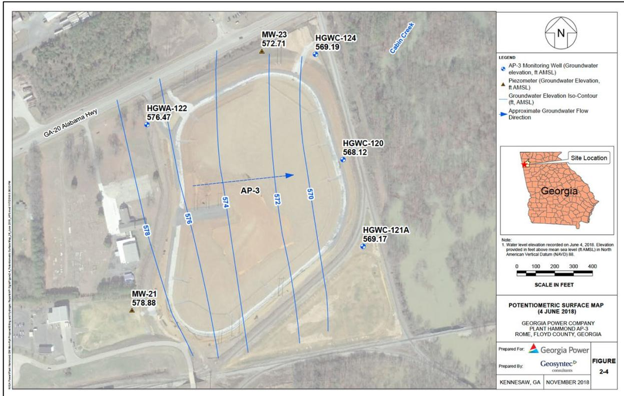
**Figure 11. Map showing eastward lateral groundwater flow beneath AP-3.**
