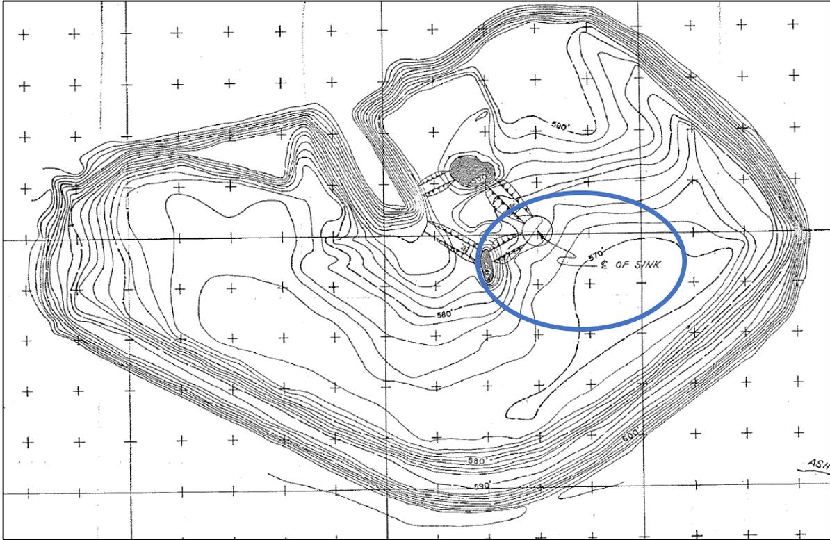
Figure 7. topographic map of AP-3 from a drawing dated November, 1979 (Part B Application pdf p. 1272). Showing the of location of a sinkhole. Added blue circle highlights the area of sinkhole.
