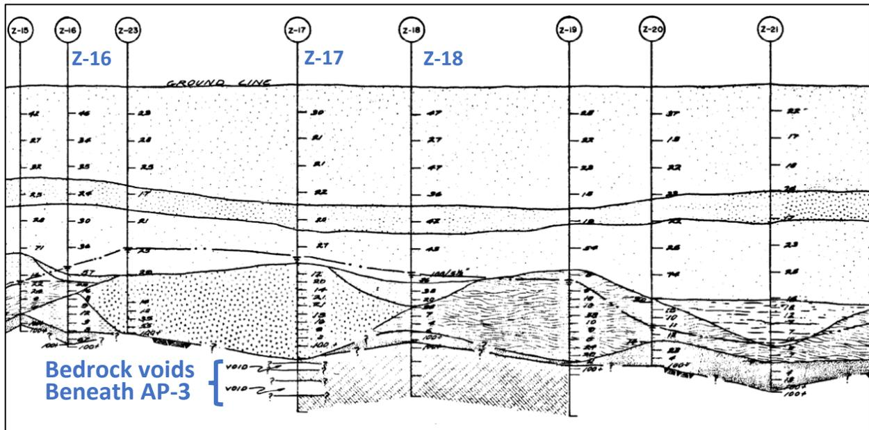
Figure 4. 1977 sketch of borings through the CCR from and underlying material, showing voids (the white spaces indicated are voids, or empty spaces the otherwise solid bedrock) in the beneath the pond that have formed from limestone dissolution that were known before AP-3 was initiated. This diagram, though not labeled, is apparently from the 1976-77 Georgia Power Company (GPC) investigation.
