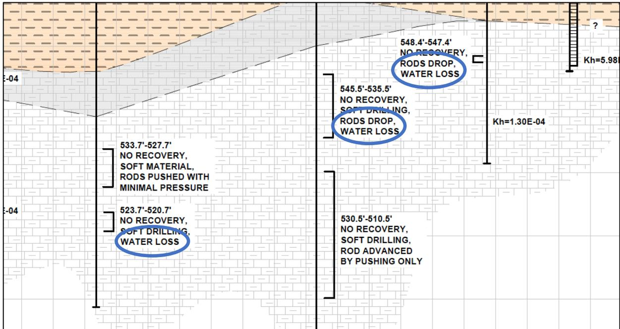
Figure 9. Part of an AP-3 cross section C-C' (Plan B Application pdf p. 35) showing three wells where drilling fluids were lost, highlighted in blue, draining away into the network of karst conduits that permeate the Conasauga Limestone beneath Plant Hammond. The hydraulic conductivity of such fractures is so much higher than the surrounding solid rock, it is generally assigned *infinite* values in numerical groundwater flow models (see references in text).
