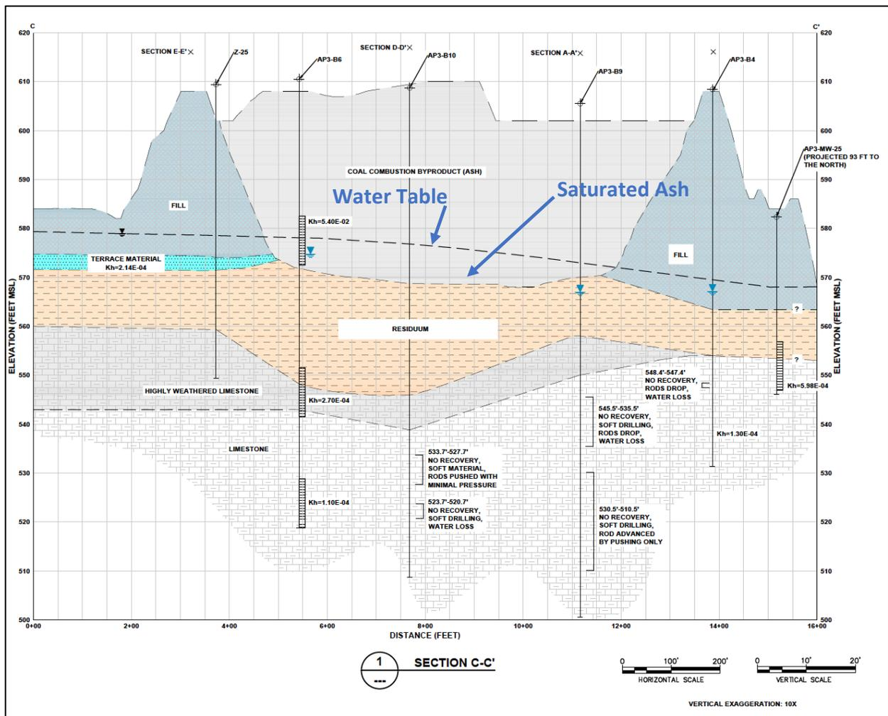
Figure 10. Cross section C-C' with area of saturated ash, and the top of the saturated zone, or water table, labeled.
