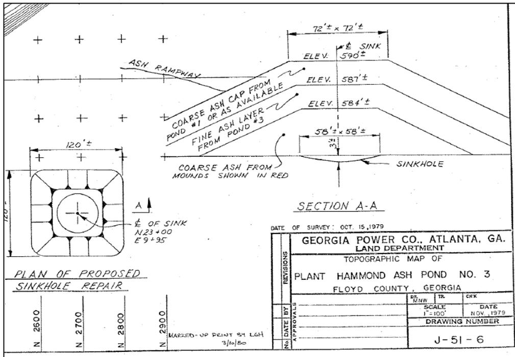
Figure 8. Details of proposed sinkhole repair for the same drawing as that from Figure 7 Indicating that the sinkhole was 58 feet in diameter (Part B Application, pdf p. 1272).
